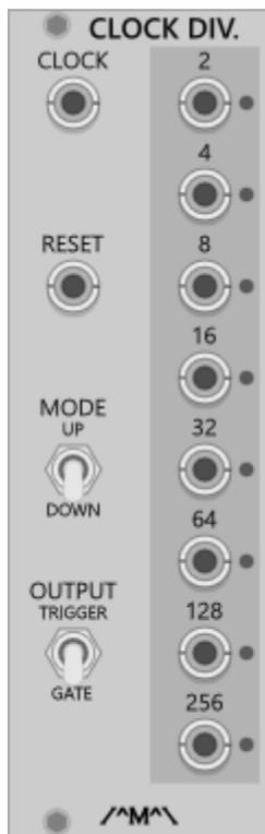
A clock/pulse divider with simultaneous outputs for division by 2, 4, 8, 16, 32, 64, 128, and 256. The divider is essentially a binary counter with the division outputs reflecting the status of each bit.
