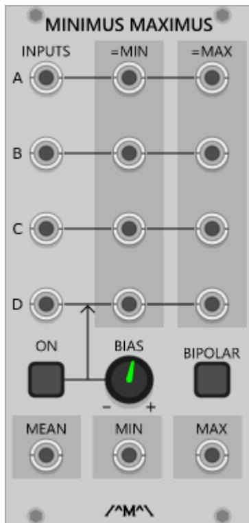
A signal processor that determines and outputs the minimum, maximum and mean (average) of up to 4 input signals along with gate signals (switchable between unipolar and bipolar values via the Bipolar button)) for each input channel indicating that the associated input is equal to either the minimum or maximum value.
