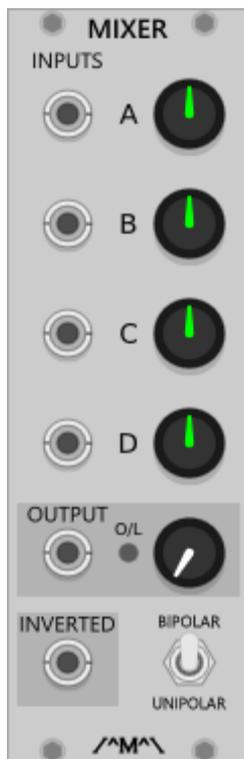
A basic 4 input utility mixer with output level control, overload indicator, inverted output and selectable bipolar/unipolar operation. The first input channel acts as a CV source if no cable is plugged into the jack.
