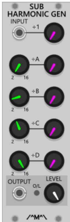
Accepts a signal from a VCO/LFO and generates a mix of user selectable sub harmonic square waves. This module works best when fed with a square wave but will function with any other waveshape.
