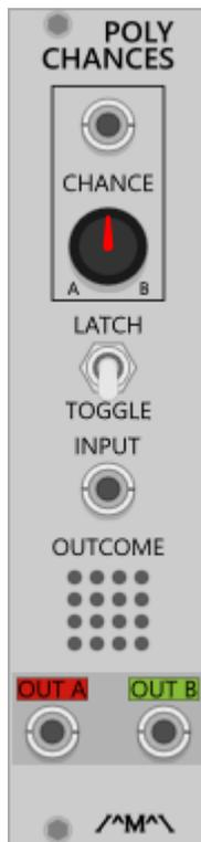
A polyphonic voltage-controlled Bernoulli gate that randomly sends gate a gate signal to either one of the two outputs.
