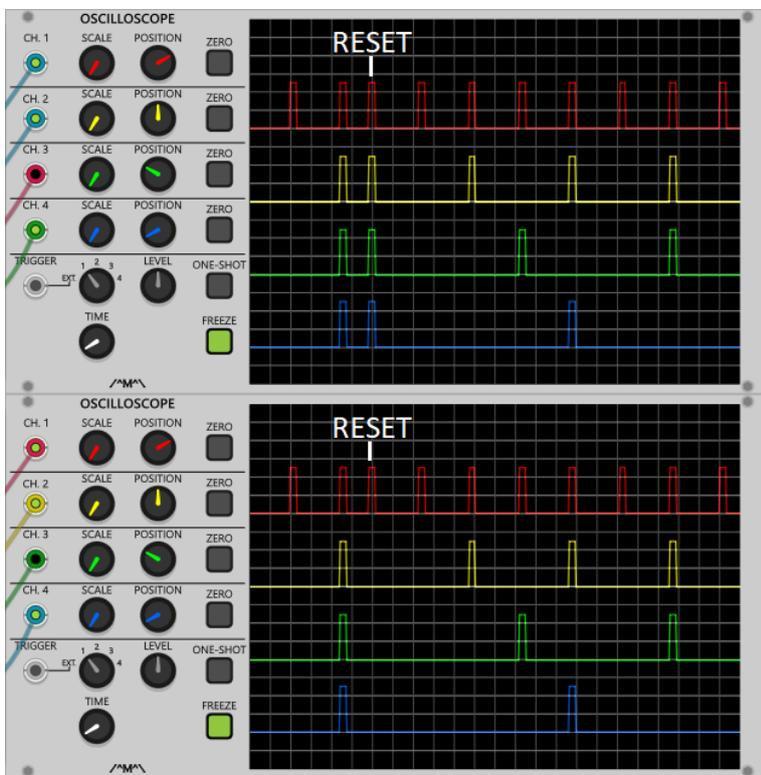
The scope image to the left shows the outputs of 4 divided clock outputs from a single clock module that were converted to trigger signals.
