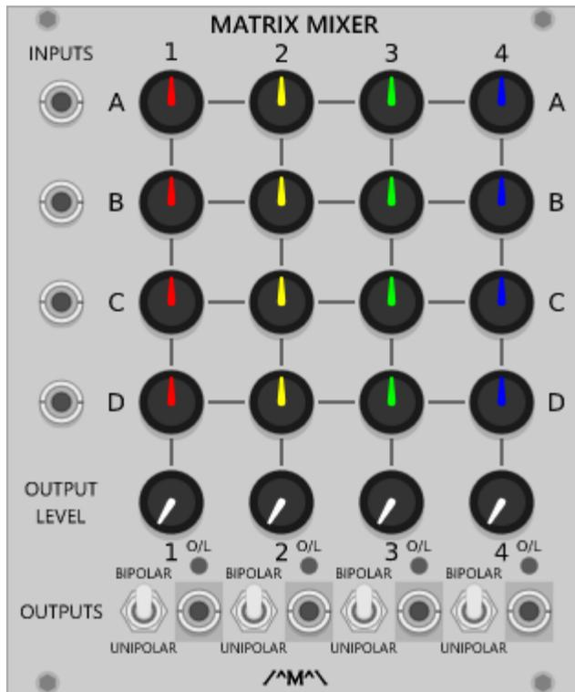
A 4 x 4 matrix mixer allowing up to 4 input signals to be independently mixed to 4 different outputs.
