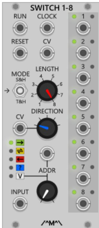
A 1 input to 8 output sequential switch/router. A signal presented to the input is routed to one of eight outputs sequentially, randomly or by voltage address depending on the chosen mode.
