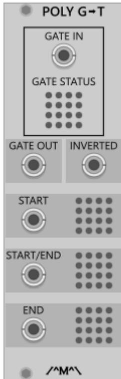
Converts any polyphonic signal into polyphonic gate and trigger signals.
