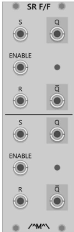
A dual Set/Reset flip flop with optional enable.
