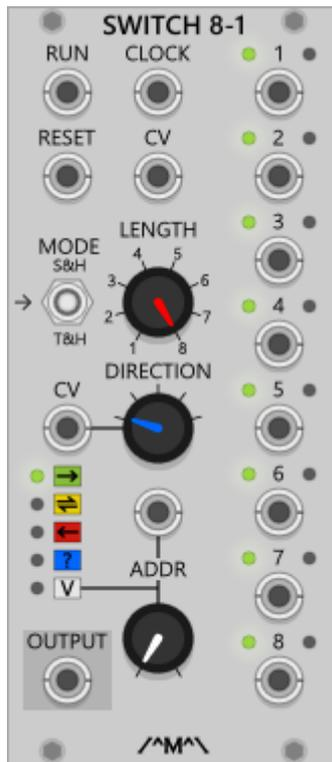
An 8 input to 1 output switch/selector. The signal present at the selected input is routed to the output with the input being selected sequentially, randomly or by voltage address depending on the chosen mode.
