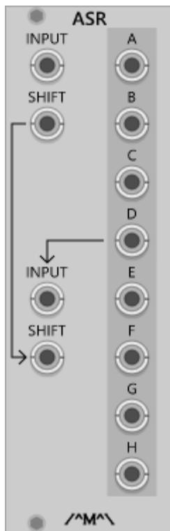
A dual 4 output or single 8 output shift register. On each the rising edge at the shift input, the signal present at each output is propagated to the next successive output and the input is simultaneously sampled and sent to the first output. The shift input on channel 2 is normalled to the shift input on channel 1 and the signal input on channel 2 is normalled to output 4 of channel 1 so that, with no cables connected to channel 2, the module functions as a single 8 output shift register.
