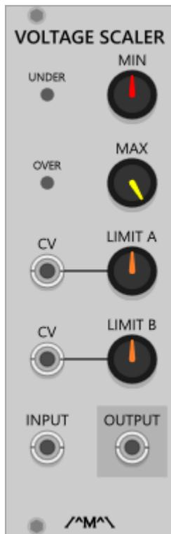
The Voltage Scaler translates input voltages within a defined range to another voltage-controlled range and can be used to re-scale and/or offset any voltage.
