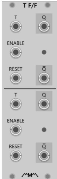
A dual Toggle (T type) flip flop with optional enable.
