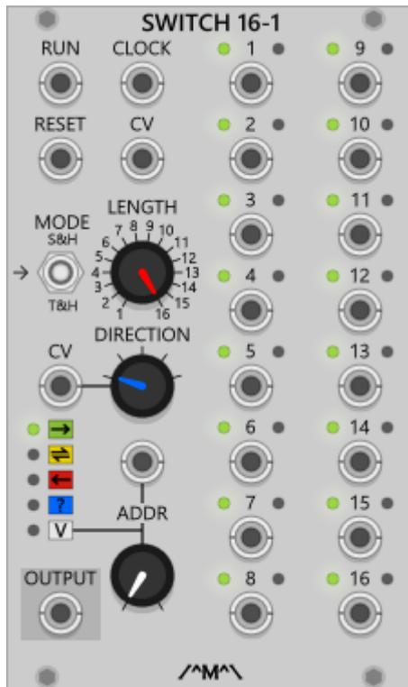
A 16 input to 1 output switch/selector. The signal present at the selected input is routed to the output with the input being selected sequentially, randomly or by voltage address depending on the chosen mode.
