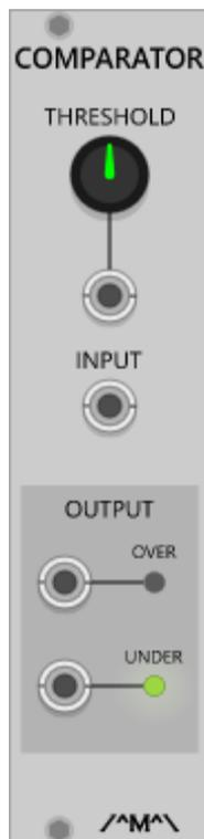
Compares the input signal with either an internal or external threshold value and outputs gate signals indicating if it is under or over that threshold.
