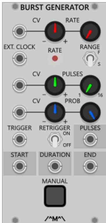
This module generates bursts of 1-16 pulses whenever a trigger is received at the trigger input.
