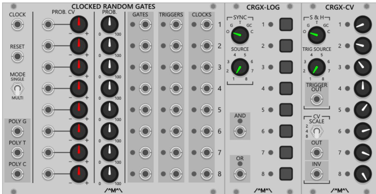
Generates a set of 8 random gate, trigger and gated clock signals quantised to the incoming clock.
