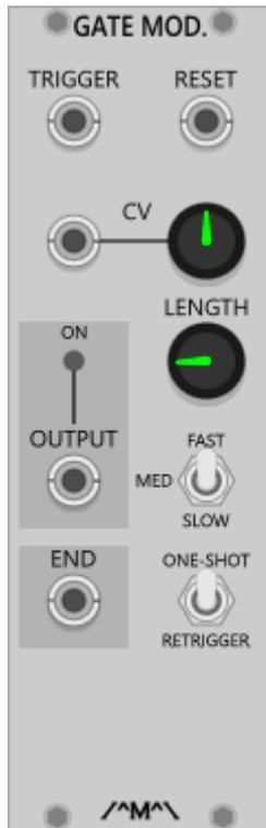
A voltage-controlled gate length modifier with the following selectable ranges:
