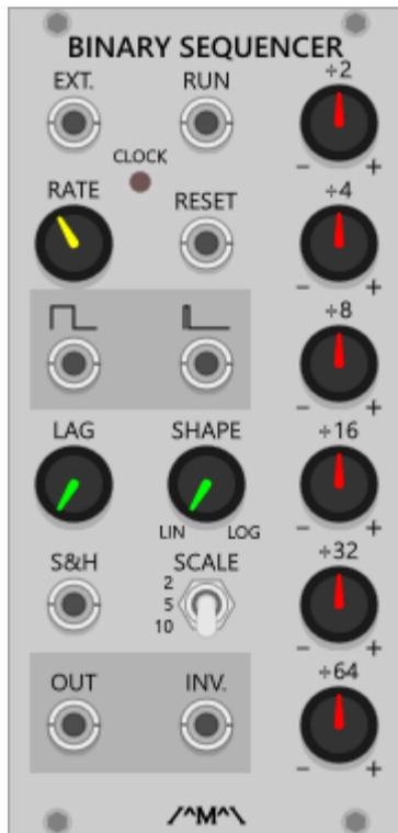
Similar to a now discontinued Frac format module, this is a binary counter based sequencer where the individual bits of the counter are mixed together in varying proportions to produce a repeating CV pattern.
