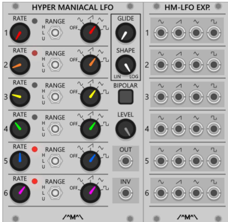
Based on the CGS Super Psycho LFO, this module expands on that concept by adding extra range, extra waveforms and an expander to break out the individual LFO waveforms.
