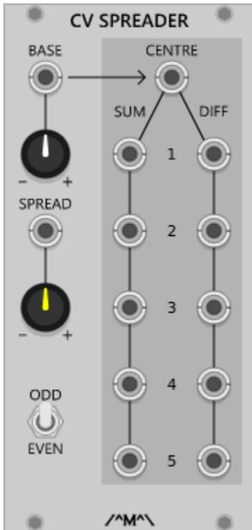
This module accepts two CV inputs, "Base" and "Spread" and creates a set of new CV values that are spread either side of the base value by an amount determined by the spread value.
