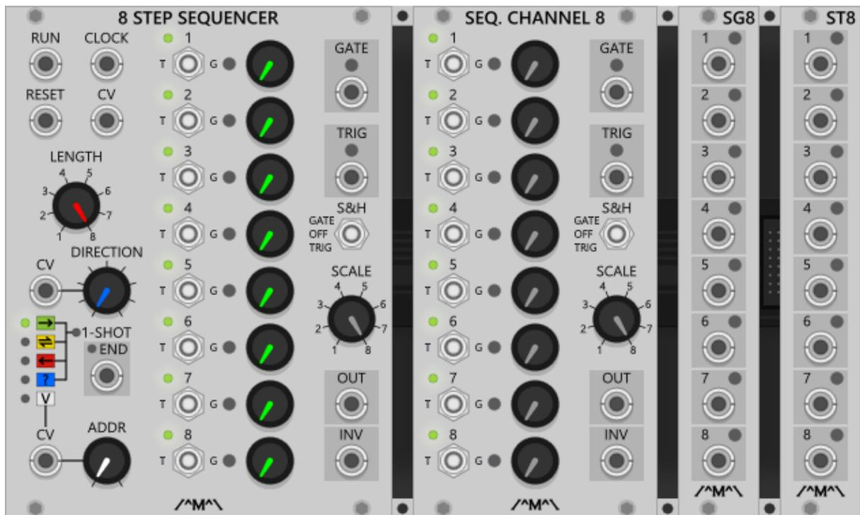
An 8-step trigger/gate/CV sequencer with voltage control over sequence length and direction, one-shot mode and built in sample & hold.
