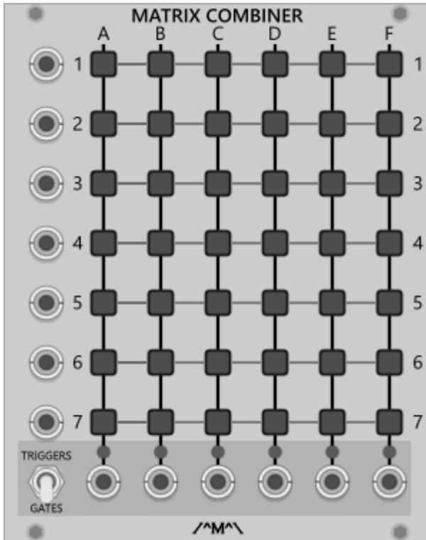
A push button matrix that allows up to 7 gate/trigger signals to be independently “OR” combined and routed to any of 6 output destinations.
