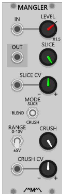
A voltage-controlled sample rate and bit depth reducer or "bit crusher" designed to make a lo-fi mess of your audio or CV signals.
