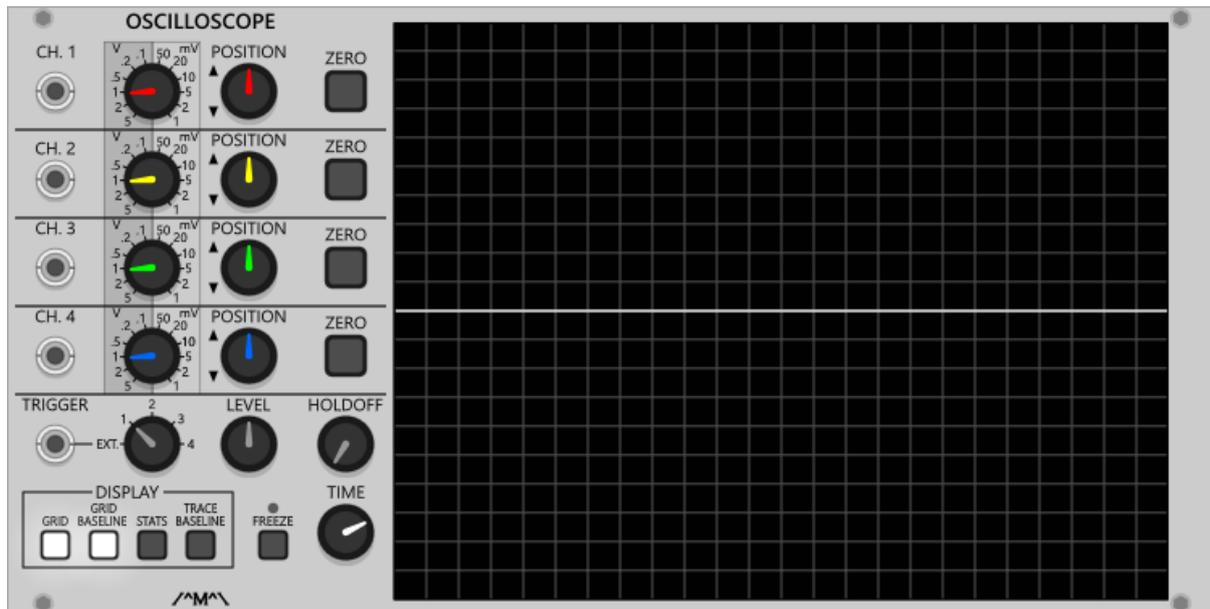
An oscilloscope with a large display and 4 independent traces. Note this oscilloscope is NOT capable of displaying polyphonic signals.
