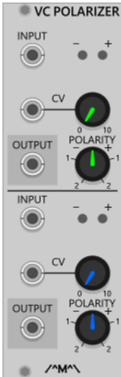
A dual voltage processor that inverts or “polarizes” the incoming signal under manual/voltage control.
