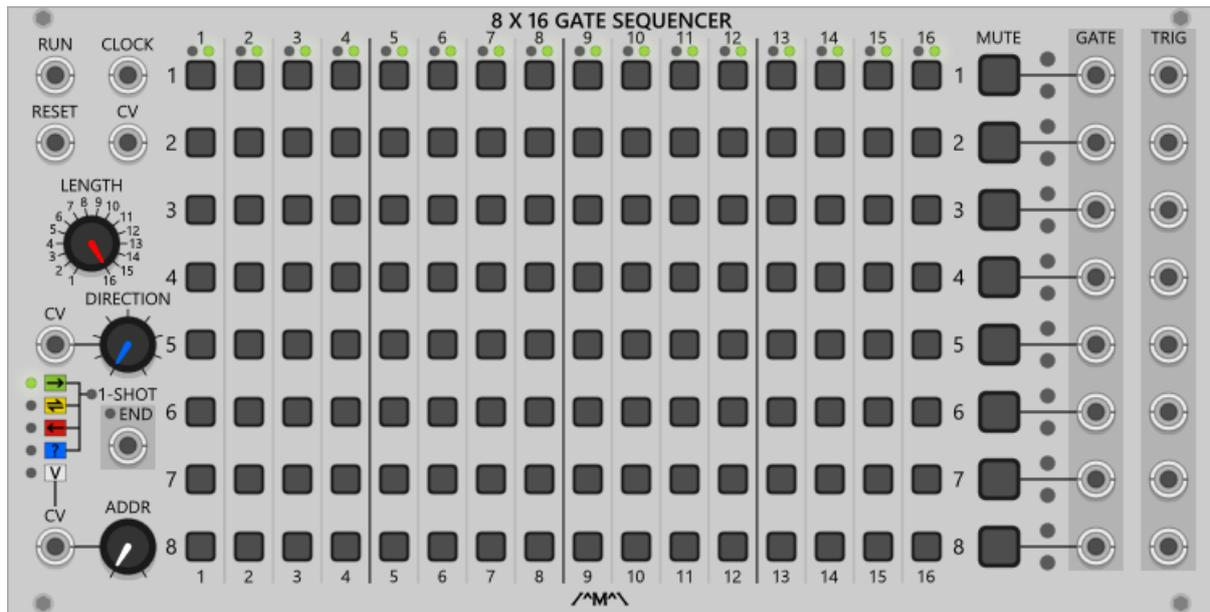
An 8-channel x 16 step gate sequencer with voltage control over sequence length and direction. This sequencer differs from the 16 Step Trigger Sequencer in that all channels are commonly clocked and addressed rather than individually.
