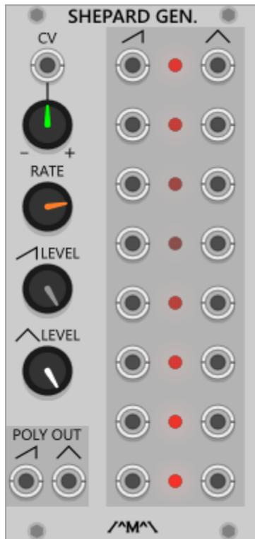
Generates a set of 8 ramp and sawtooth signals appropriately phased for generation of Shepard tones (tones that sound like they are continually rising or falling) when coupled with 8 VCOs and VCAs. Slower modulation rates and linear VCAs work best for this effect.
