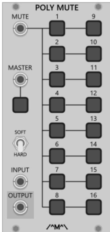
Muting of individual channels within a polyphonic signal with a Master Mute that operates on all channels within the signal and switchable response (hard/soft) for instant processing of control signals or fast but pop free muting of audio signals.
