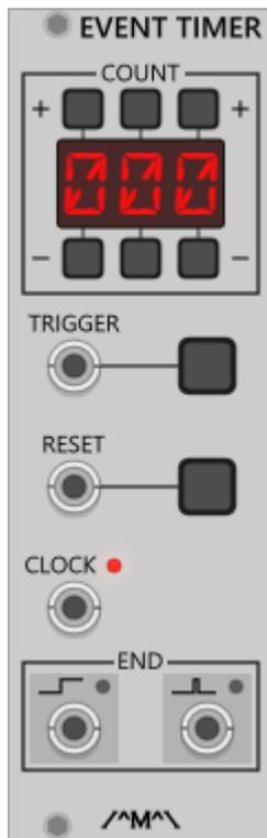
A triggered count down timer that outputs a trigger and gate at the end of the count.
