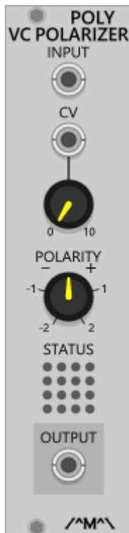
A polyphonic voltage processor that Inverts or “polarizes” the incoming signal under manual/voltage control.
