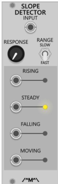
The slope detector generates gate pulses from a CV input based on whether it is rising, falling, steady, or moving.
