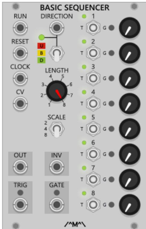
A single basic 8 step trigger/gate sequencer with voltage control over sequence length and direction. For a more fully featured version of this sequencer see the 8 and 16 Step Sequencers.
