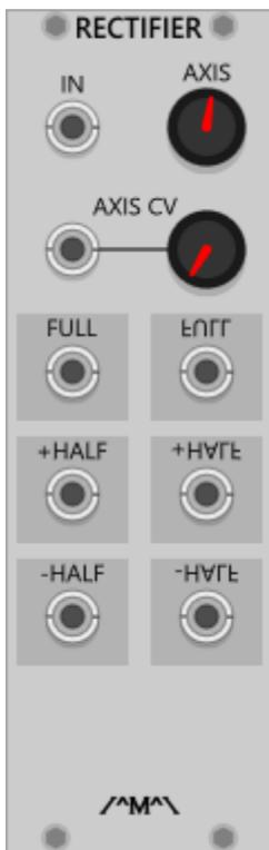
A precision rectifier offering full wave, and both positive and negative half wave rectification. The input signals are rectified around a user settable and voltage controllable axis.
