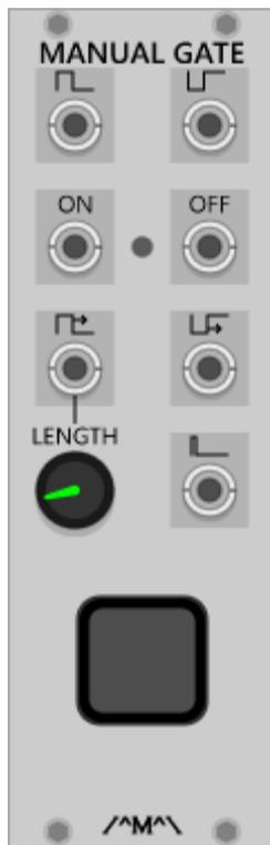
A manually triggered gate generator offering a number of simultaneous gate and inverted gate outputs.
