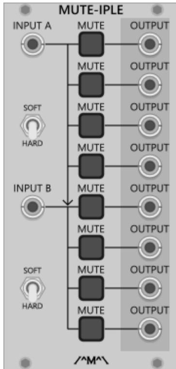
A dual 4-way/ Single 8 way mutable multiple. The top input is normalled to the bottom input creating a 1 to 8 mutable multiple.
