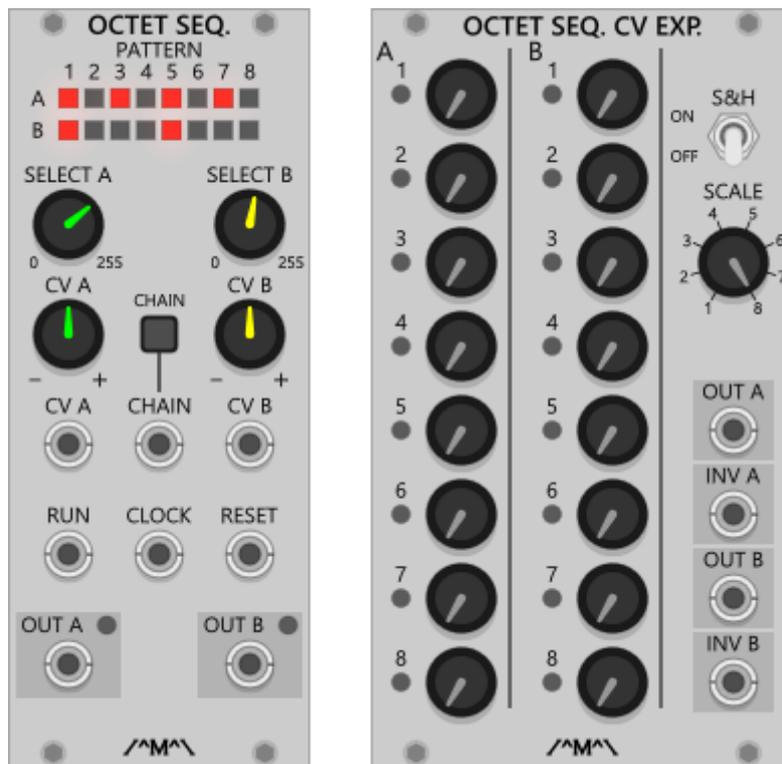
A two-channel trigger sequencer based on the principal that every 8-step pattern can be represented by an 8-bit binary number or “octet” and hence, any integer number between 0 and 255 inclusive.
