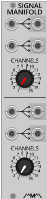
The Signal Manifold replicates a mono/poly input signal into a selected number of channels in a poly output signal. There are two independent sections with two separate, but commonly controlled, inputs and outputs per section.
