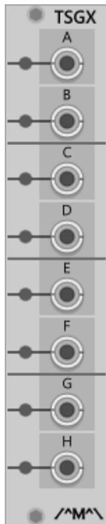
An expander that adds 2 gate outputs for each channel if the 8 and 16 Step Trigger sequencers.
