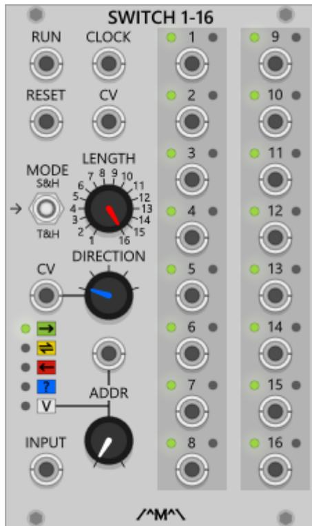
A 1 input to 16 output sequential switch/router. A signal presented to the input is routed to one of eight outputs sequentially, randomly or by voltage address depending on the chosen mode.
