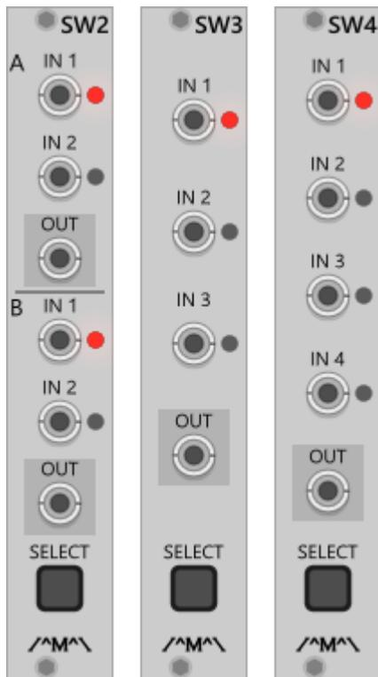
Manually operated “select” switches. The Select button sequentially connects each input to the output in turn with each successive press.
