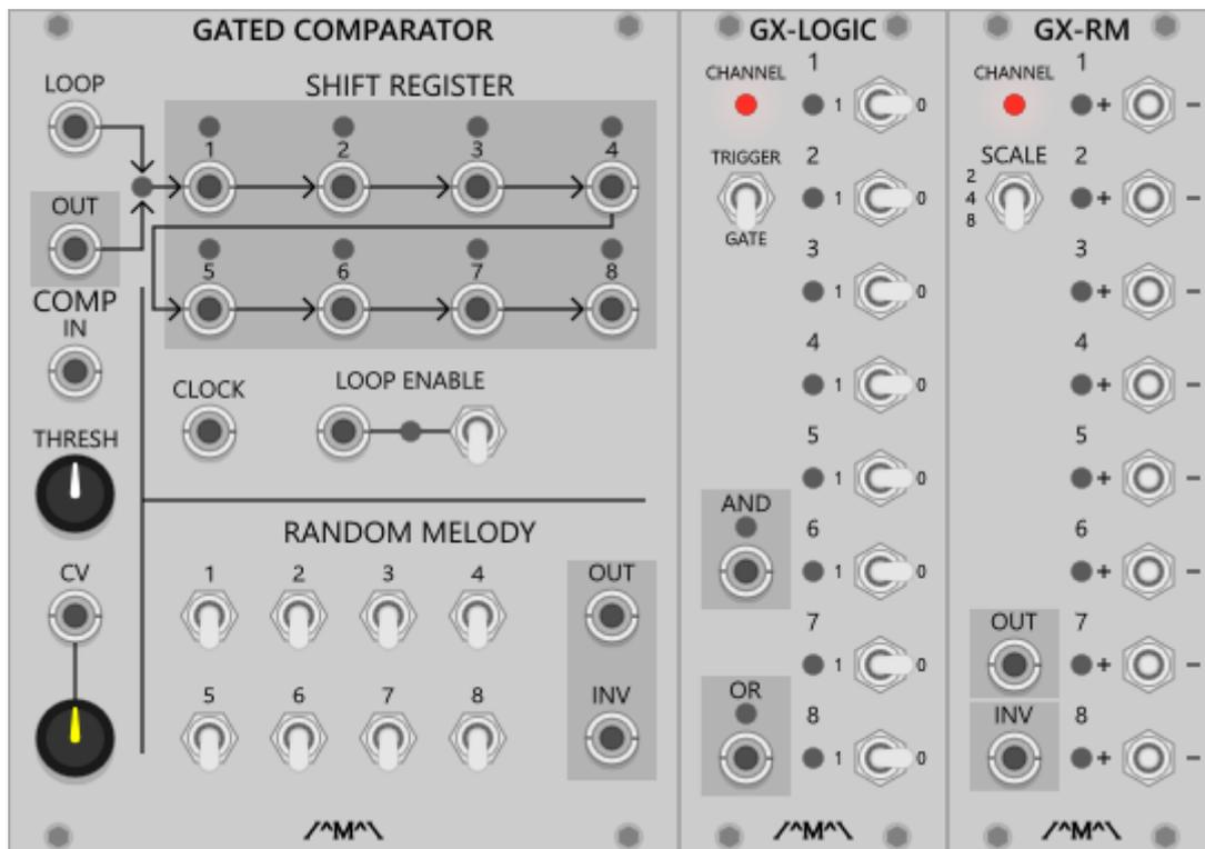
The gated comparator is a binary shift register fed by a comparator and coupled to a basic "digital to analogue" converter which can be used to generate Random sequences.
