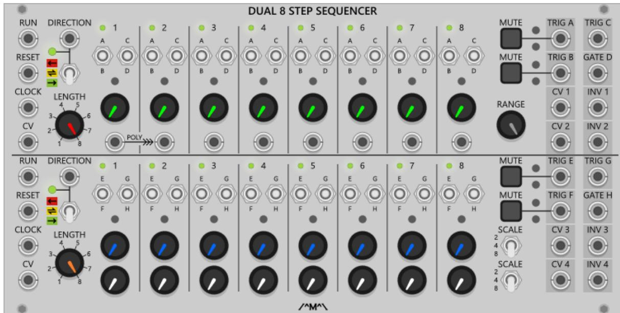
A dual 8 step trigger/gate sequencer with voltage control over sequence lengths and direction along with individual inputs for each step on one channel.
