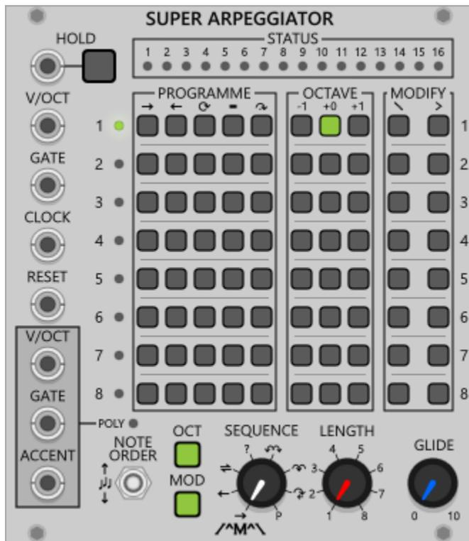
A complex arpeggiator that accepts polyphonic chord signals from a keyboard or sequencer and applies various patterns to the notes before sending them sequentially to the outputs.
