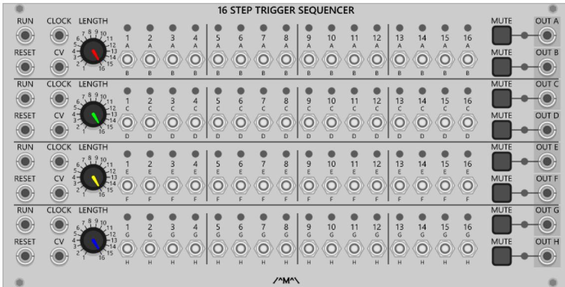
A set of four 16 Step trigger sequencers in a single panel each with voltage control over the sequence length and two independent outputs.
